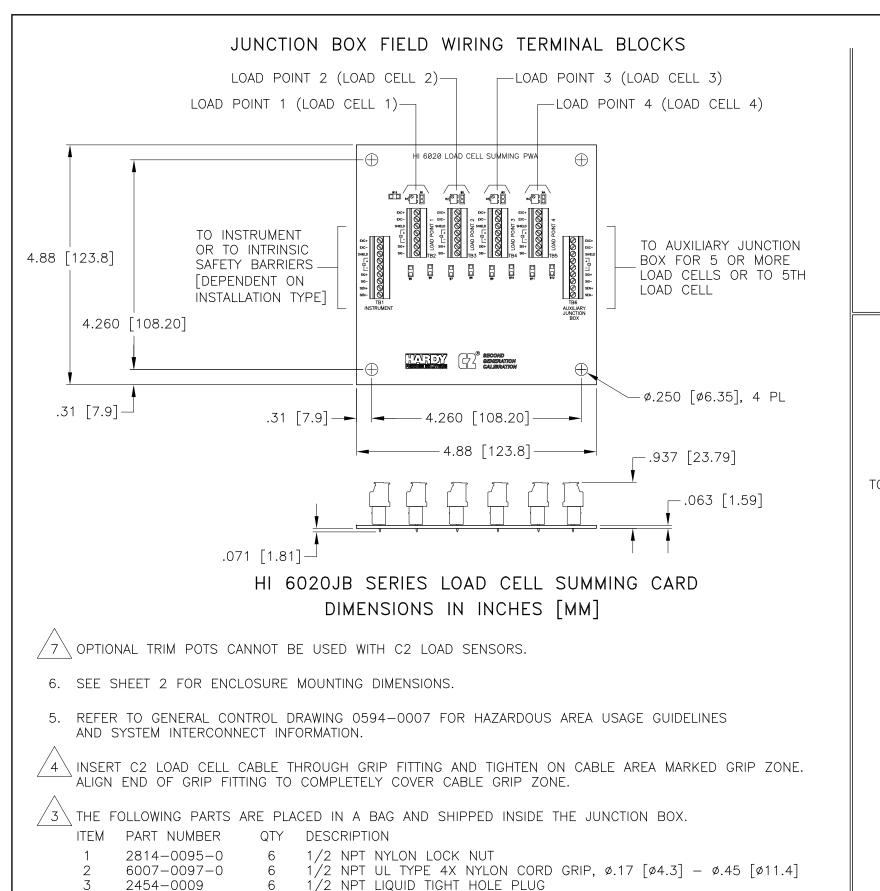
2. USE HARDY PROCESS SOLUTIONS CERTIFIED LOAD CELL CABLE MODEL NO. C2 CABLE [PN 6020-0001-0].
